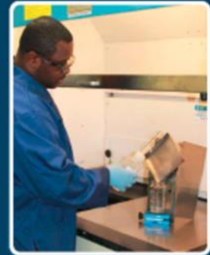
Nonvolatile residue removal efficiency test
